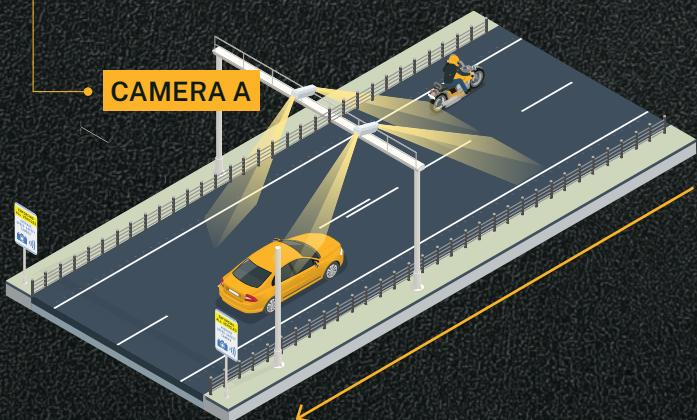
The vehicle's speed between CAMERA A and CAMERA B is then calculated.
